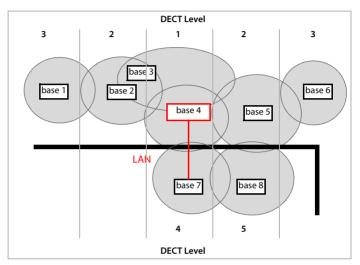
**Configuration:** Mixed scenario. The base stations of the cluster are separated by a firewall. The overlap area may be large enough for handover and dynamic channel selection but not for synchronisation. Therefore the synchronisation between one base station on each side of the firewall takes place via LAN. The other base station are synchronised via DECT. As the LAN master must be on DECT level 1 the base station 4 is used as LAN master.
